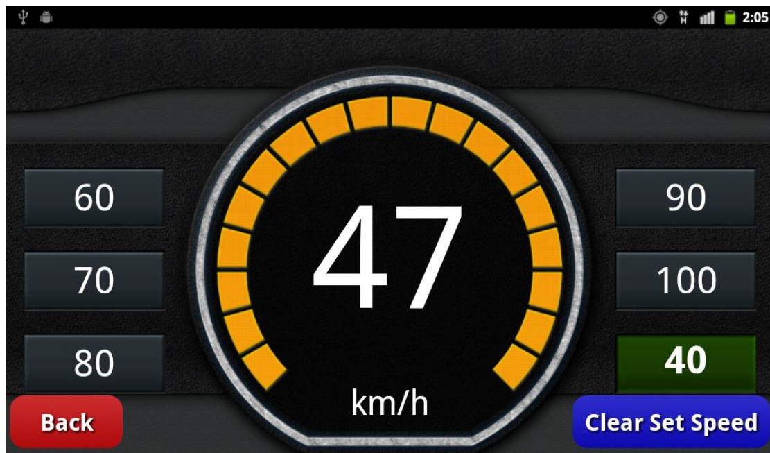
FIGURE 5 – SPEED ASSIST – WARNING “ALERT ABOUT TO SOUND” AND CURRENT SPEED SET TO 40KM/H
