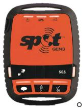
The -SPOT has 6 buttons and 8 LEDs.
